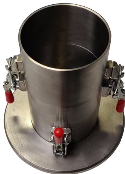
TML Proctor/Fagerberg mould with extension
