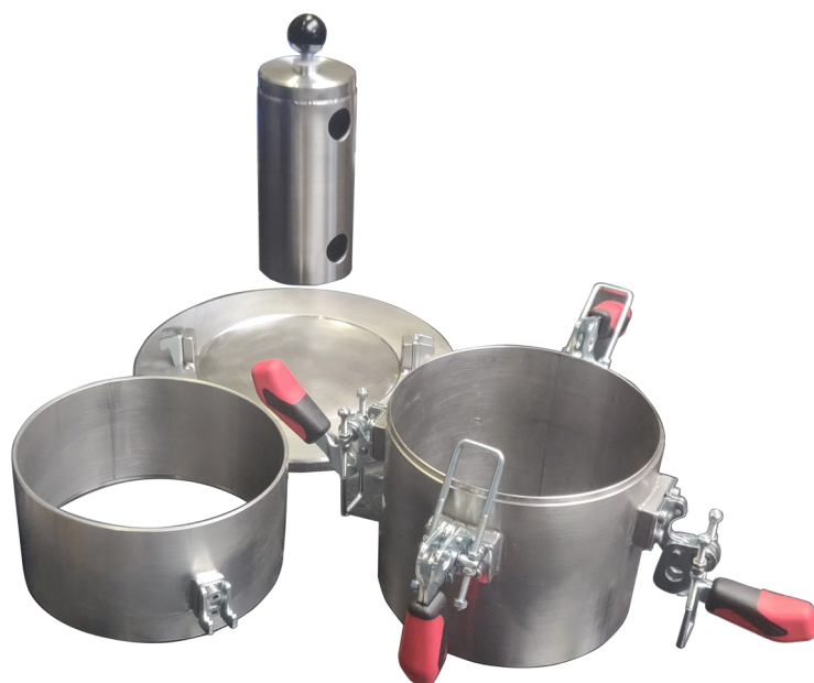
TML Proctor/Fagerberg equipment disassembled
